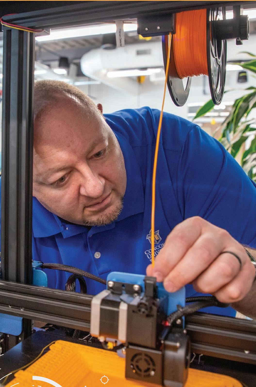
Dr. Mike Litman loads filament into the extruder on one of the direct drive 3-D printers in the new makerspace at Concordia University Wisconsin.
